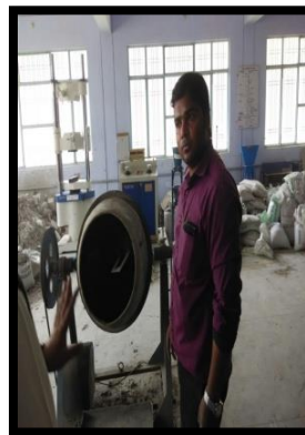
Mixing of Concrete by Mechanical Mixer. Preparation of specimens.
